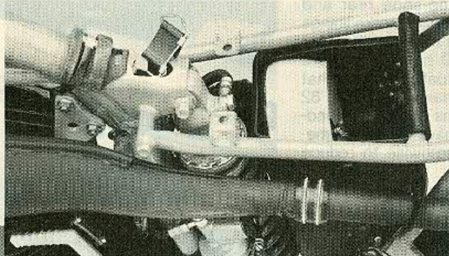
1983's most important changes include a new shock body and reservoir, airbox and removable frame section.
