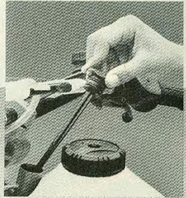
The black dipstick makes reading the oil level difficult. Frame oil capacity is 3.2 quarts.
