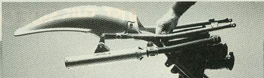
The rear frame section—including the airbox and stinger/silencer—unbolts easily to allow access to the rear suspension system.
