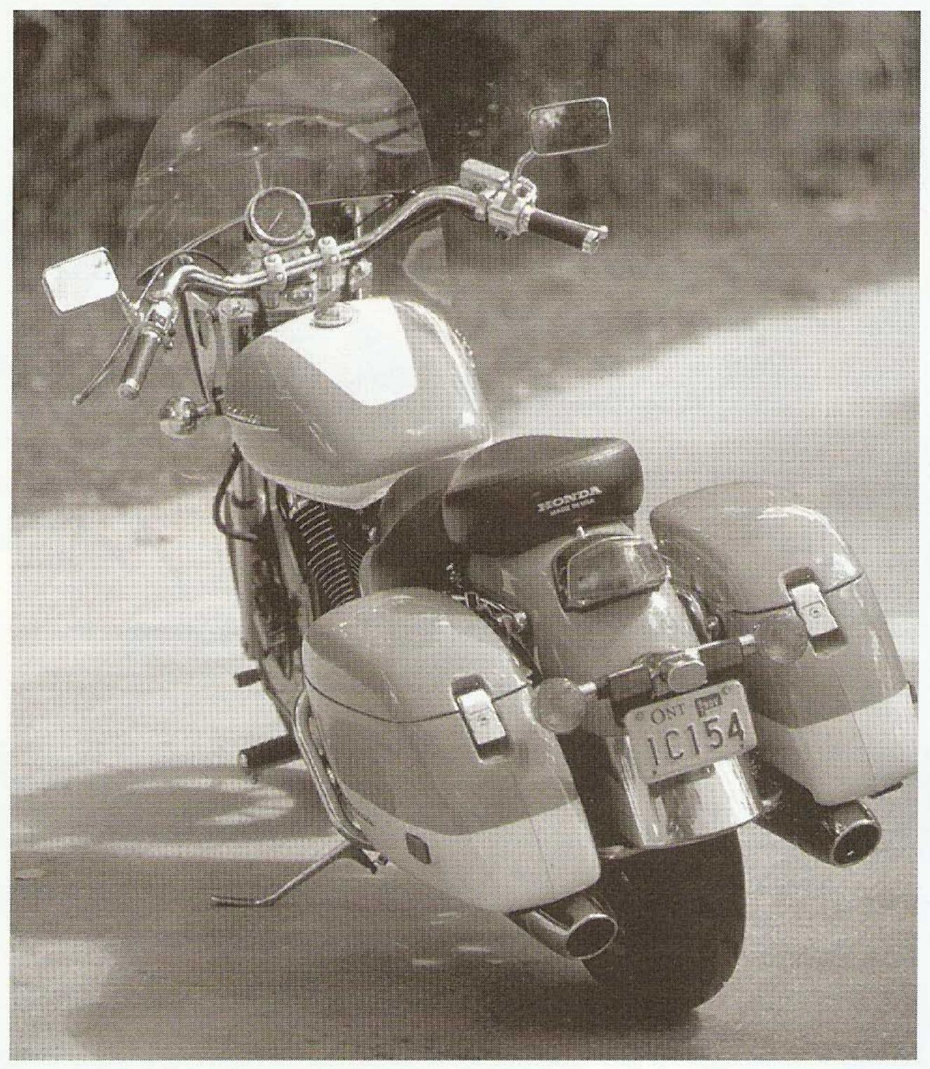
ed springing and damping of the new shocks offer a vast improvement. The suspension action has a slightly bouncy feel, but it can tolerate heavier loads and is quite free of the painful harshness that plagues the standard ACE. The swingarm on the Tourer has been braced for greater strength, and the shocks are angled differently.
