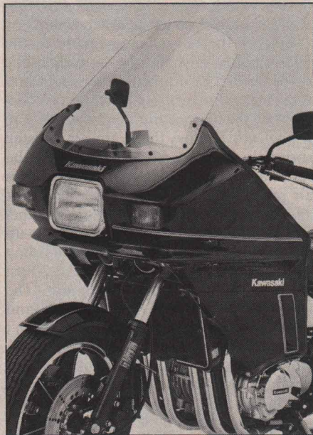
Kawasaki's fairing is huge. It provides lots of wind protection and storage room. It also traps engine heat around the rider's legs. Big halogen headlight provides good lighting.
