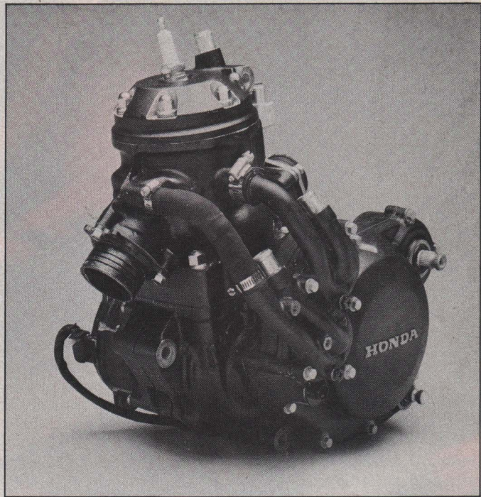
Water cooled RC250 engine only weighs 48.5 lb. full of gear oil. But the difference in weight of stock CR250 (56 lb.) isn't much when the radiator, water and lines are added.
