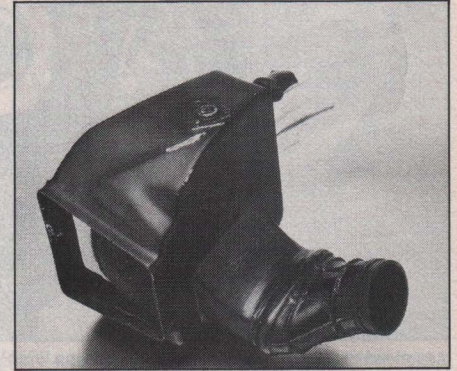
Airbox uses a large foam filter, Rear fender extension is pop riveted to rear of box.
