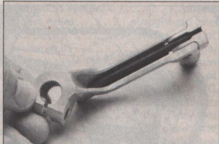
Three different length aluminum shift levers are available to factory riders. Two different styles of end pieces are also offered; the ribbed unit shown is preferred for mud races, a rubber covered model is usually used for drier races. A rubber band is used for a return spring and changed every two races.
