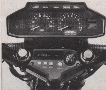
Sabre's instrument panel serves up an impressive array of facts whether the rider wants them or not. Tripmeter, clock/stopwatch, fuel gauge, temperature gauge and warning system all use LCDs.
