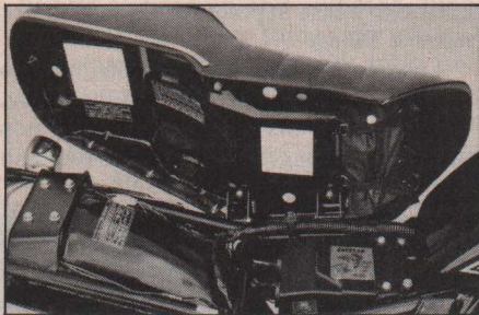
Tool kit stows nearly under bottom of seat, along with usual collection of info and warning stickers.
