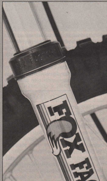
The new Fox Forx sport giant 44mm stanchion tubes and forged aluminum triple clamps and sliders.
