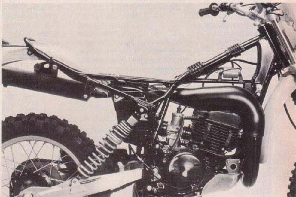
The PE uses an RM frame modified slightly to accommodate such items as a skid plate, waterproof airbox.
