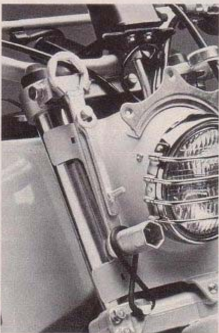
With this tool you can change a plug, adjust the chain or bar, remove either wheel, the seat or tank.
