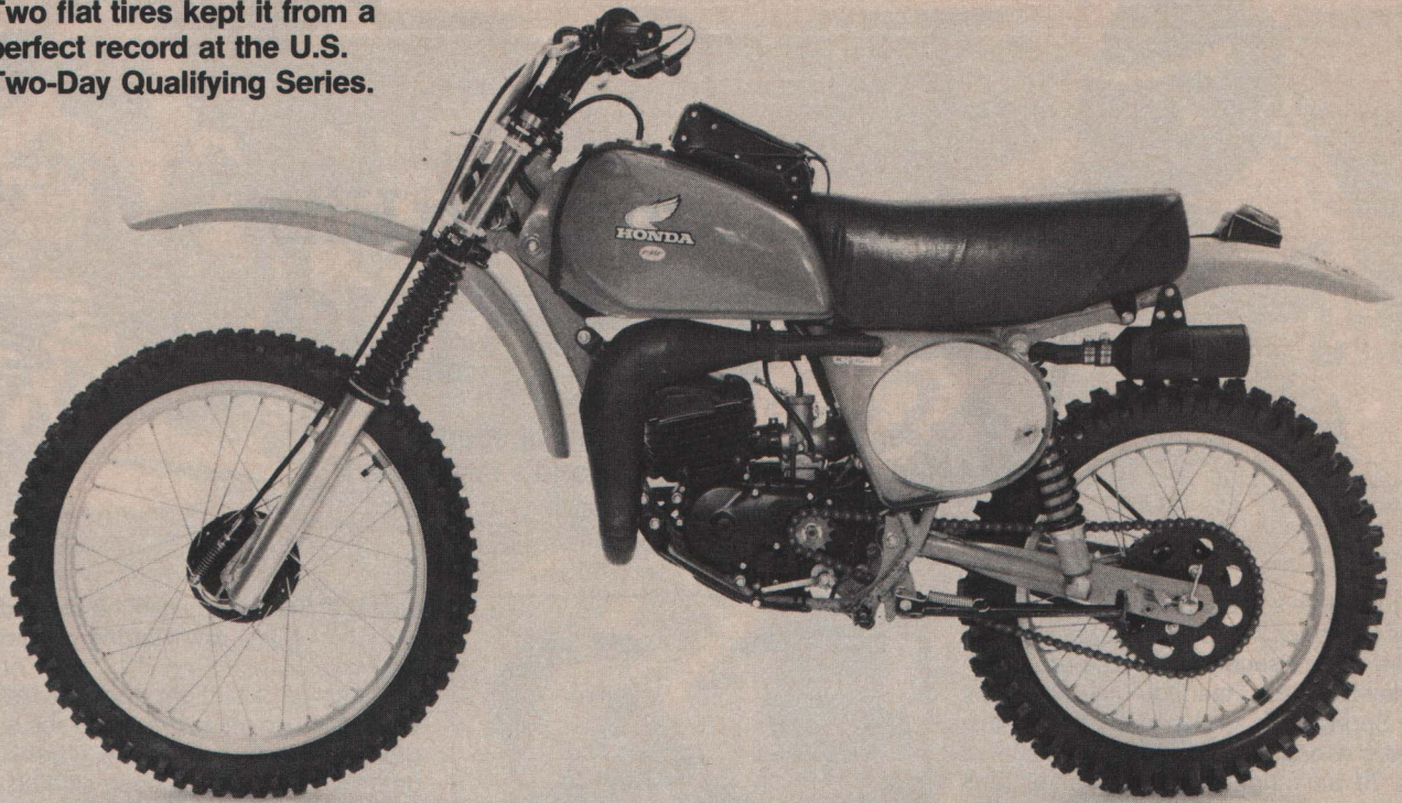
The air box and numberplate required much modification to accommodate the high pipe. Note cutaway on countershaft cover for quick access to the front sprocket.
