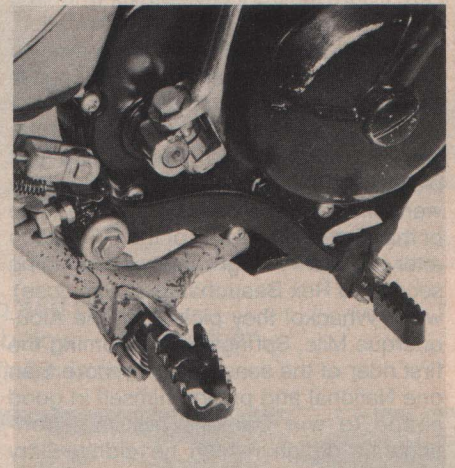
A folding brake lever is rarely damaged by rocks or branches. A rubber band helps the brake lever return.
