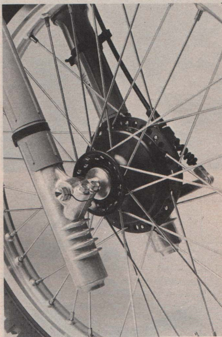
And up front: this slight-looking conical brake allows quick stops—given sufficient lever pressure.
