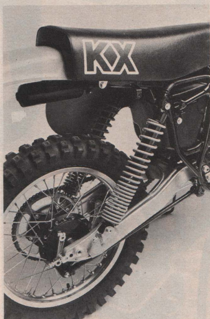
Oh-so-soft primary spring windings, aluminum swing-arm (with die-cast ends), full-floating brake stay.
