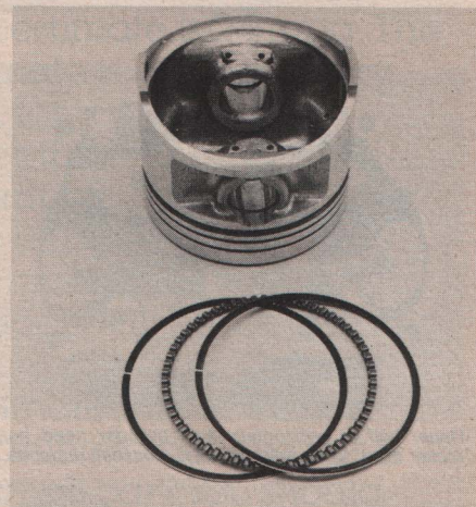
Honda 185 aluminum piston (sans compression rings) and three-piece, automotive-style oil control ring.
