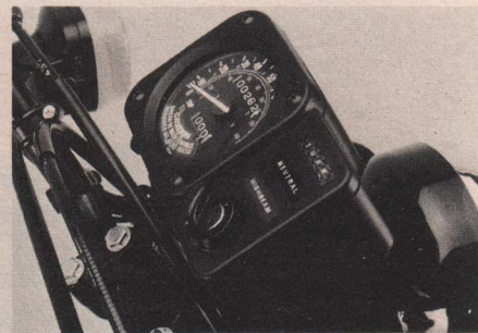
This shoe box instrument pod houses the speedo and odometer, ignition lock and three warning lights.
