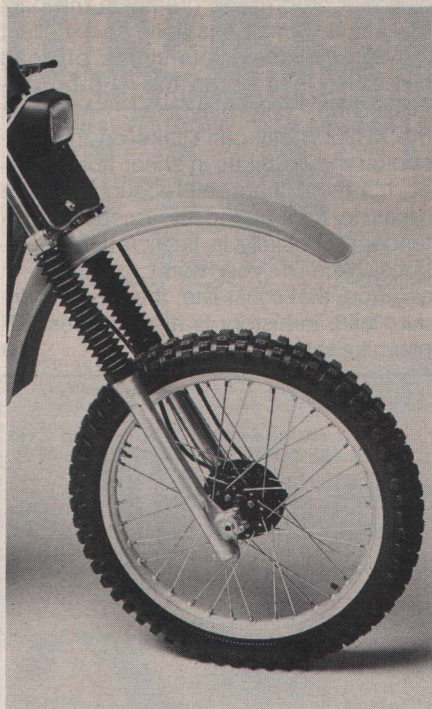
New front end sports many changes, including larger fork tubes, tapered roller bearings and air caps.
