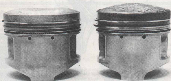
The 750 Seca piston is two millimeters larger in diameter than the 650 Maxim slug. It has a wider skirt for increased thrust area and a greatly reduced crown height.
