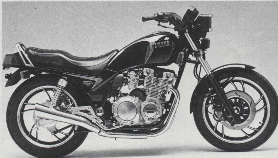
Yamaha's anti-dive unit adds little unsprung weight and features a check-valve system that is adjustable.
