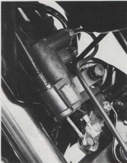
The front brake cylinder is hidden behind the headlight. Unfortunately, brake feel got lost in the move.
