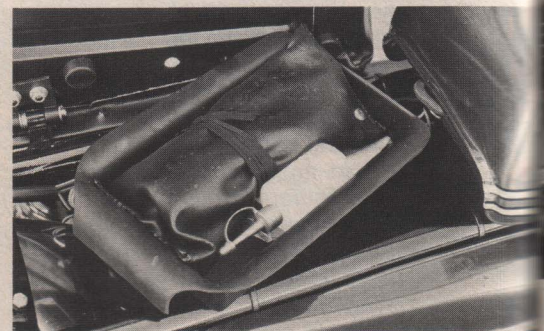
Under the hinged seat, there is a lift-out tray containing a tool-roll and a squeeze bottle for chain lube.
