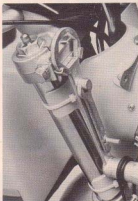
Detail and refinements include an improved multi-purpose wrench and air-assisted front suspension.
