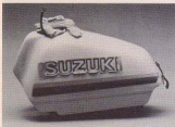
PE-T's 2.8-gallon tank replaces the N's 3.2-gallon tank and slops gas from your navel to your knees.
