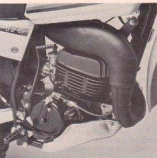
Following the lead of Team Suzuki, the factory has updated the engine and extracted 22.38 bhp.
