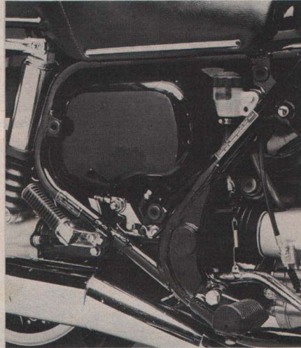
One liter has been added to the Wing's fuel capacity. Beneath the tank is a common shock absorber air valve.
