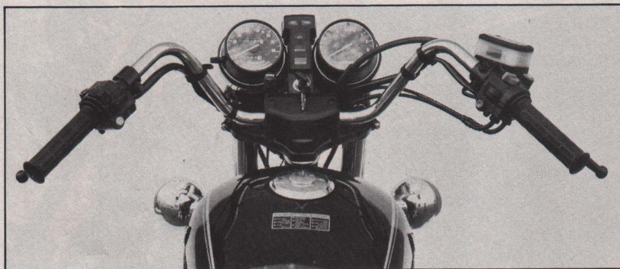
Cruise-controller's view: new locking gas cap, dashboard and wheelbarrow bars
