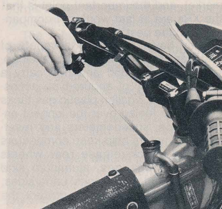
The XR500 engine is a dry-sump design; engine oil is stored in the frame backbone and front downtube.
