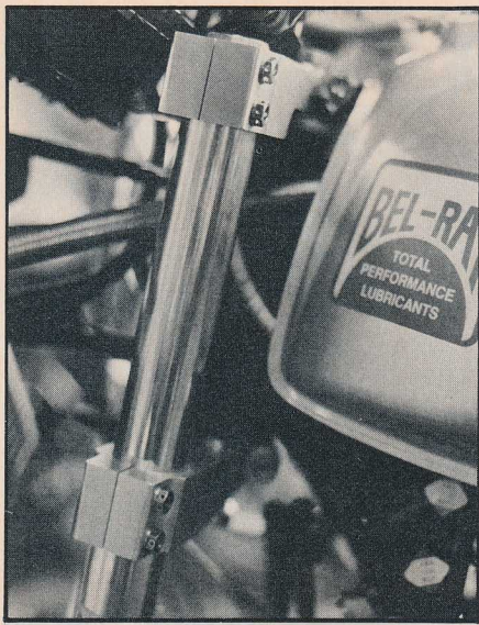
Special triple-clamps, produced for varying geometries, are machined alloy with much relieving on undersides.
