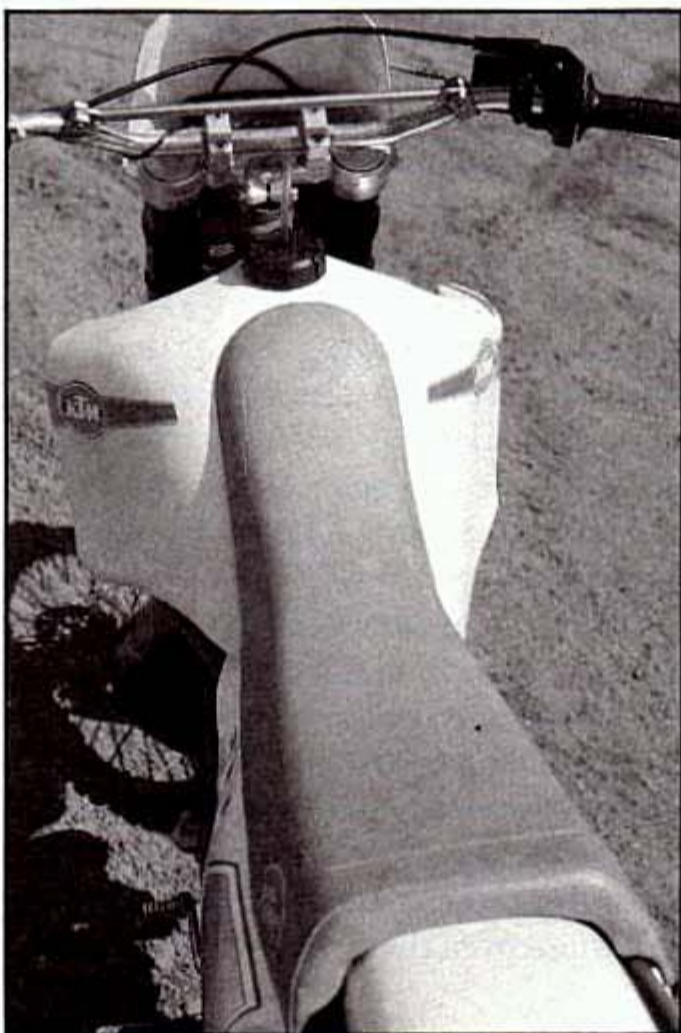
KTM's good ergonomics owe much to its seat And nothing to the wide fuel tank.
