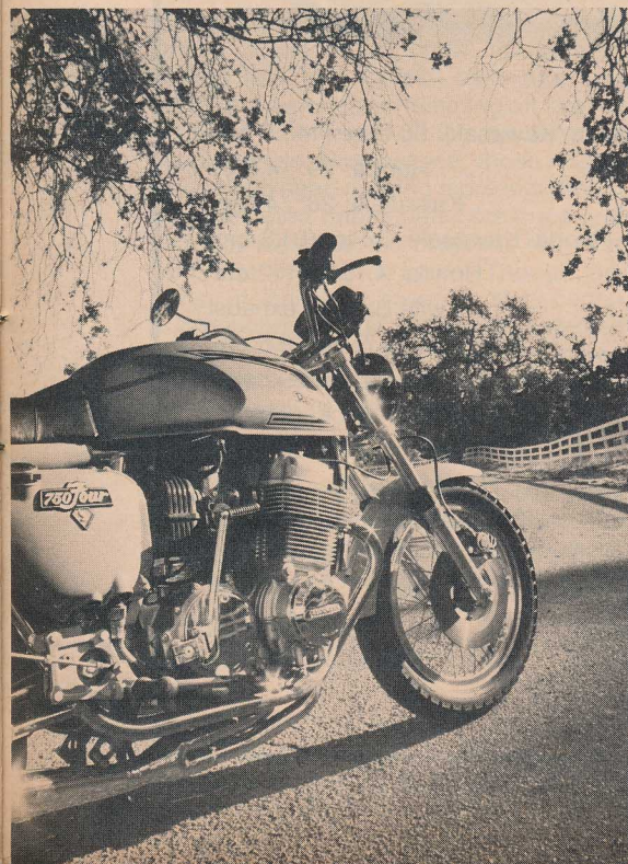
On the Rickman two-seater the large cap opens the steel gas tank under the fiberglass cover. Three screws (one at rear, two at filler cap) attach the shroud to the gas tank. The steel tank holds 4.1 gallons.
