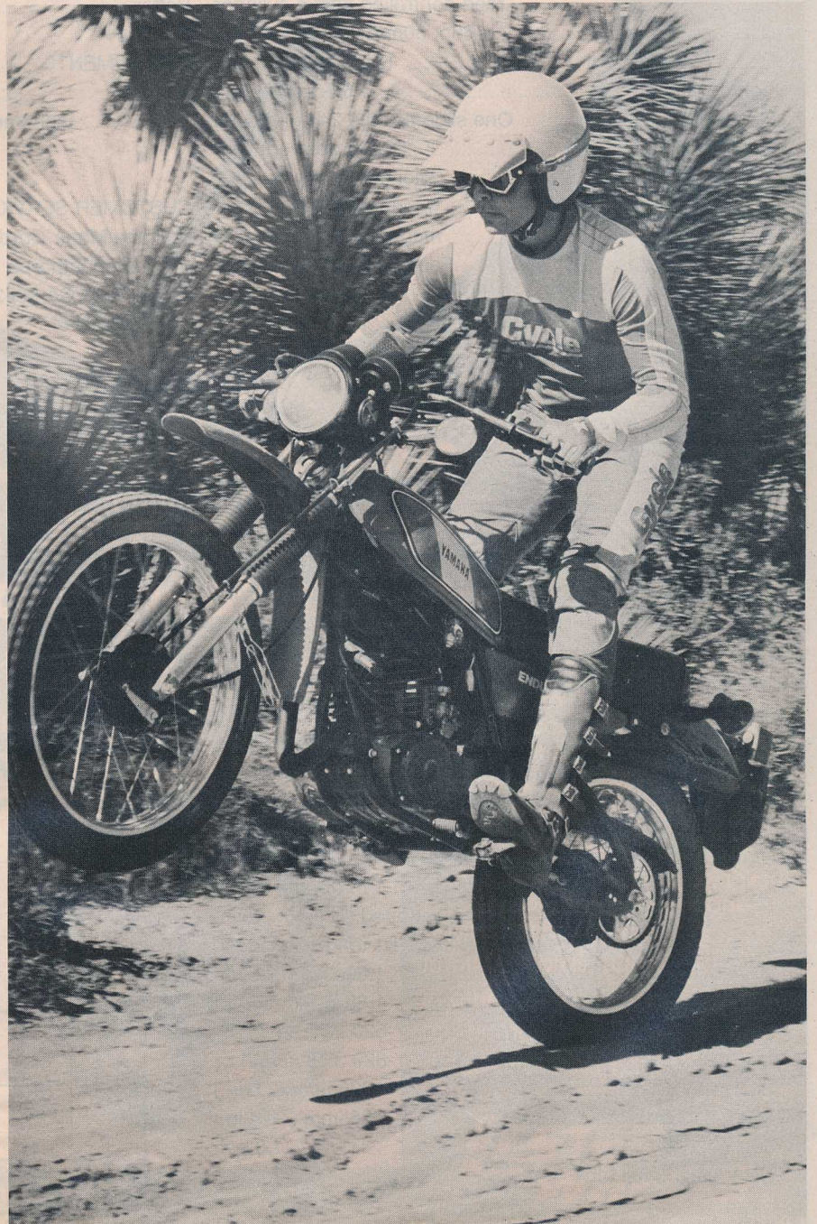
The swing-arm member rising from the axle adds to rear-end rigidity. Spark arrestor/muffler is effective.
