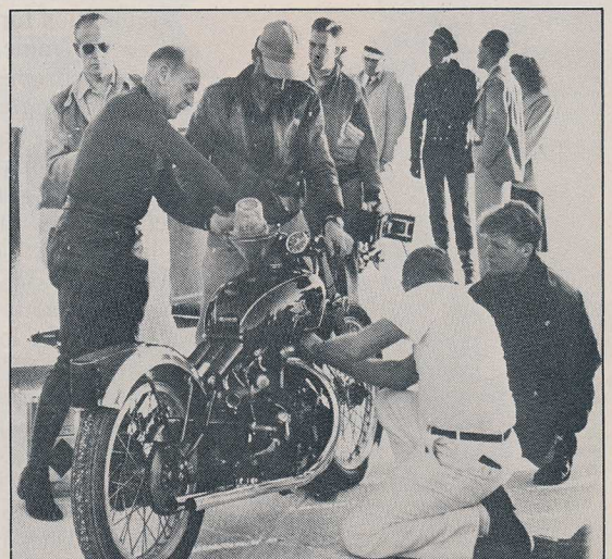
At Bonneville, preparing for the run before the run. For the record, the Vincent used was a Black Lightning, the tuned and stripped version of the road-legal Black Shadow.
