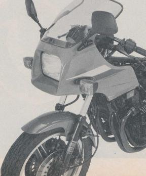
GPz fairing bolts to the frame and is made of ABS plastic. Forks have 37mm stanchion tubes and include anti-dive fittings. psi for normal street use to 28 psi for racetrack or very hard canyon riding. The shock air fitting is mounted on the frame just below the right side panel. The damping adjustment knob is also below the right side panel, with minimum rebound damping selected by pushing the knob in and maximum damping selected by pulling the knob out.
