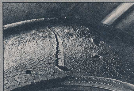
The Goodyear 1997A with newly-developed compound #825 was the preferred tire at Laguna, but the rubber seemed to stick to the asphalt better than it adhered to itself.
