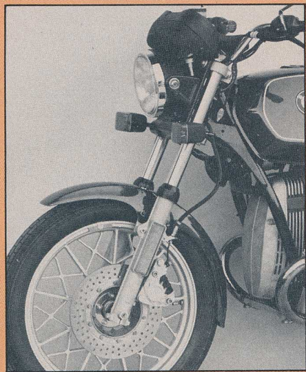
The new R65 front end: lighter forks with less travel; all-hydraulic brake system, double-piston caliper; one-piece mount for headlight, instruments and signals; cast-in reflector holders and a stylish front fender.
