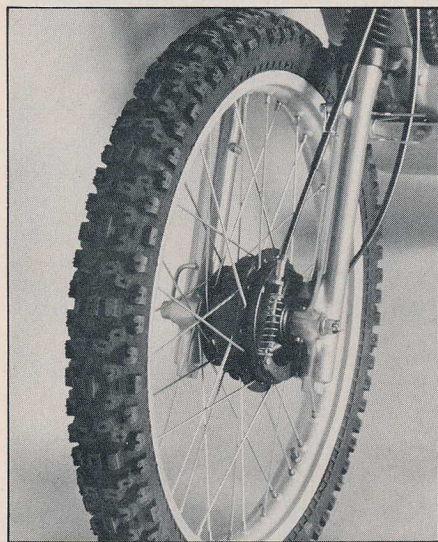
Leading axle forks use tapered shoulder on both sides. Brake lever looks exposed, but didn't suffer damage during test. Sturdy return spring protects against mud clogging the works.
