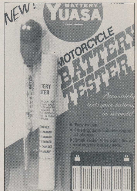
An example of a simple, inexpensive hydrometer. The small balls inside the suction tube are different densities. The more balls that float in the battery's electrolyte, the greater the specific gravity of the fluid, and that indicates more charge.
