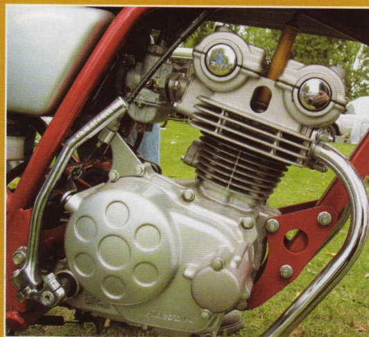
Not a sports moped as such, Dave Jefferson's Honda CB50 attracted lots of attention. "It's a grey import made in around 1998," he told me, "and is basically a C110 replica." The Japanese market dohc four-valve engined bike makes 5.6ps at 10,500rpm, and is rumoured to be the most powerful 50cc road machine in mass production. Dave also owns a TY50, two FS1-Es, an XS650 and a Honda CB400F.
