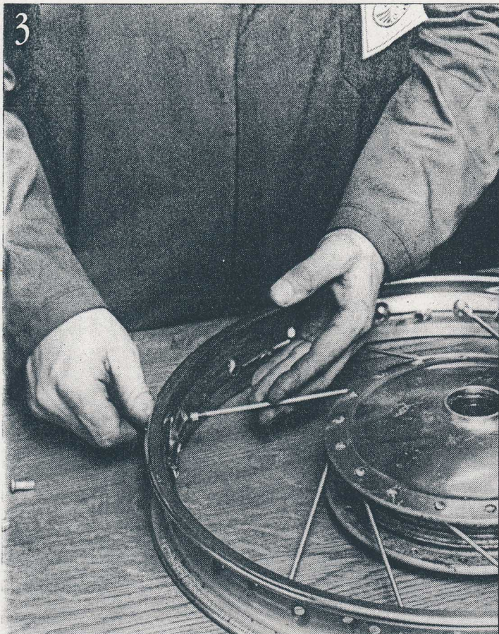
3 A twist of the hub will show you just how the spokes are supposed to line up.
