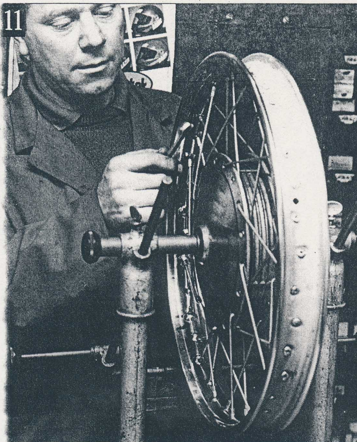
Final spoke tension is checked by ear. Each spoke should give off the same note when tapped.
