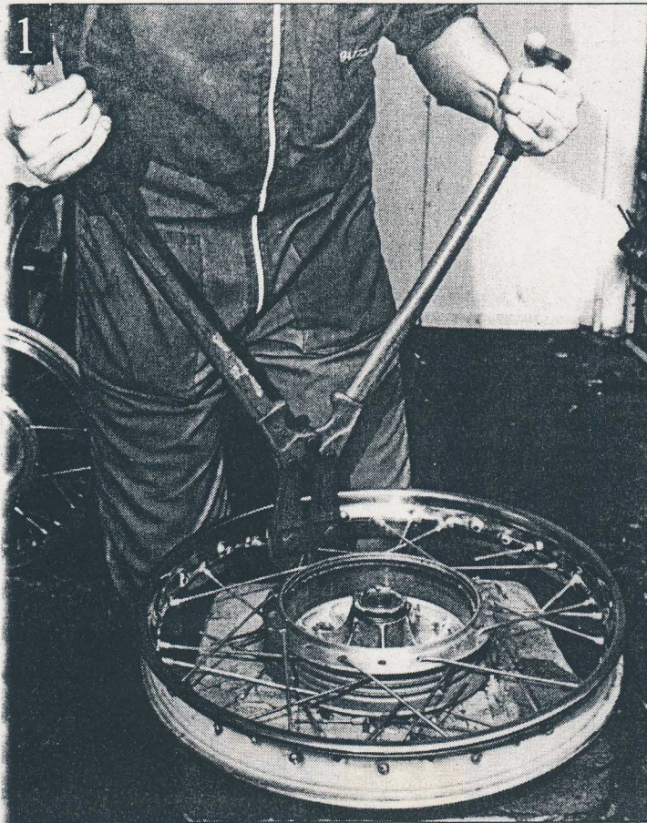
1 Chop the hub out after you've made a careful note of the lacing pattern and any offset.
