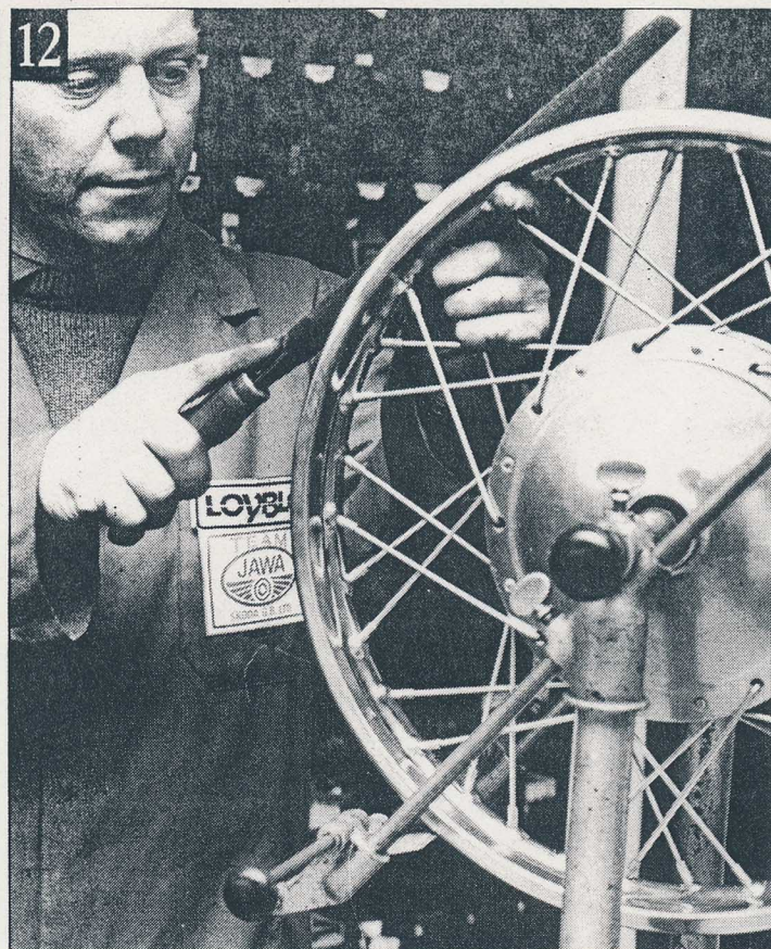
If spokes have been cut to right length, few will protrude past nipple and require filing.
