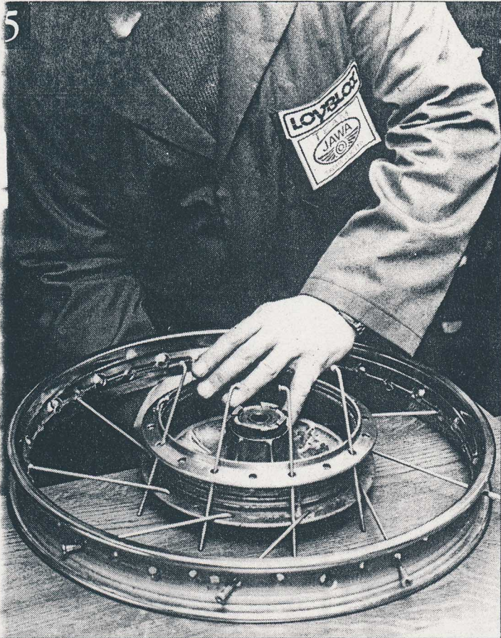
5 Turn over to insert the 'inner' spokes on the other side of the rim and then ...
