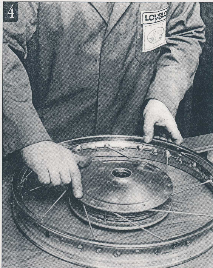
4 Once you've got a few nipples on, twisting the hub round will show you how it goes.
