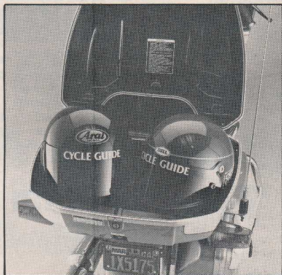
Travel trunk rated for 20-pound capacity Or two helmets with room to spare.
