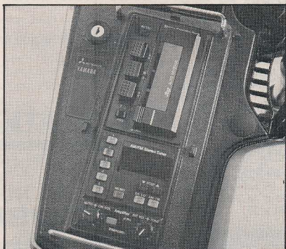
Ignition key locks sound unit in place The radio locks itself on channel.
