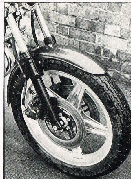
Above: Comstar wheels are all aluminium, tyres are tubeless, discs are from the GL1000 but the caliper is all new having greater leverage ratio.
