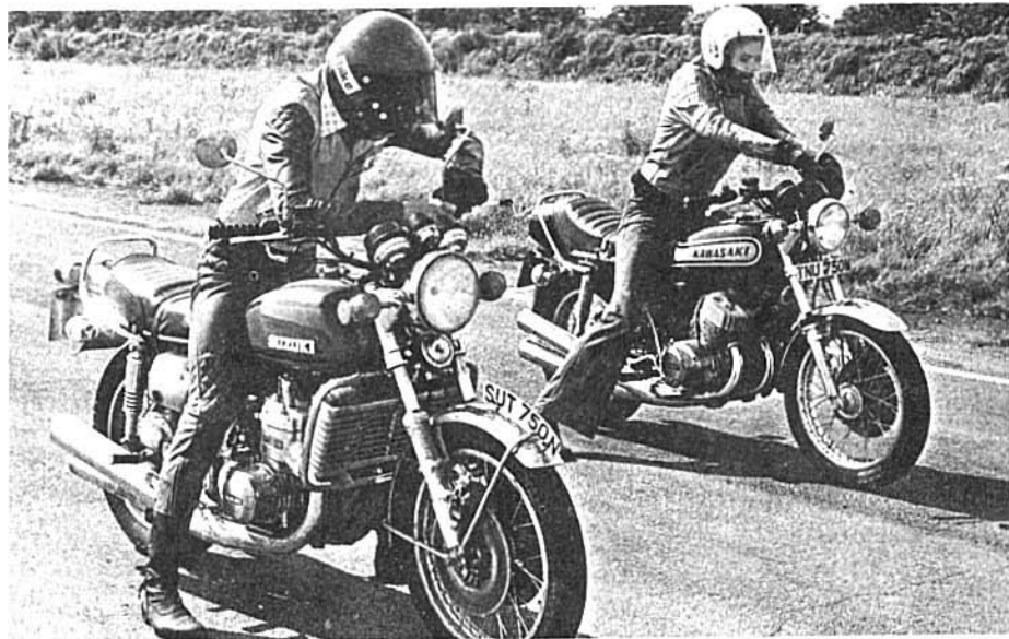
Bike's destruction testing team at it again. Four or five drag starts for the standing 1/4 mile plays havoc with clutch adjustment. The Suzu survived but it was all too much for the Kawasaki, who's clutch gave up the struggle the following day.
