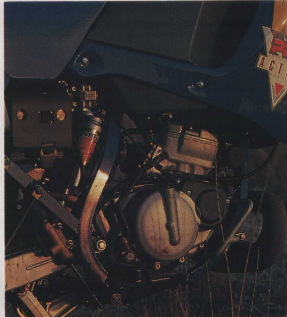
Electronic powervalve on ex-Mito engine gives W8 a useable mid-range and a healthy surge at 7000rpm
