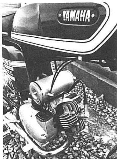
Above left: Carb for rotary valve engine nestles behind right hand side cover.
