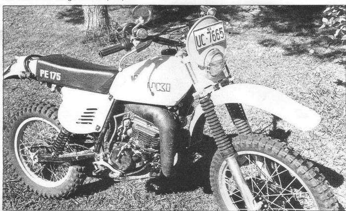
ost 175 enduro bikes are a compromise as far as engine design is concerned. They are either stretched 125 engines, or scaled down 250 engines. Neither of these approaches is ideal for power, although they are ideal for cost: it is easier to tool up to produce a 175cc barrel, piston and crank which fits onto a 125 than it is to begin from scratch and build a good 175 in the first place.
