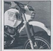
**ABOVE** Front suspension is more than adequate: the forks give less travel than the TT, and use smaller tubes, but they do the job with ease. When the tank is full you might find it necessary to pump them up a few psi. We can see owners fitting twin quartz halogen lights to really finish the bike off. Love the hand protectors, fork boots and fat front guard (just what you need in the desert . . . ).
