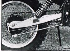
Swingarm is an extruded aluminium section which is far stronger than any other type of alloy swingarm construction. The shocks are fine for all but the best riders, but aren't rebuildable. There are two damping settings and three spring preload settings. Fully floating brake works well.
