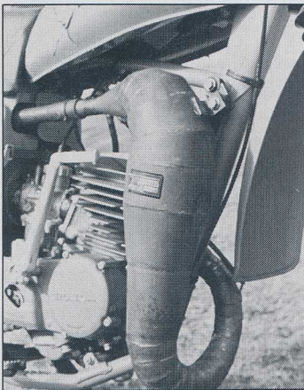
ABOVE: You can see the complexity of the new pipe. It uses the old tail piece and silencer off the original pipe.
