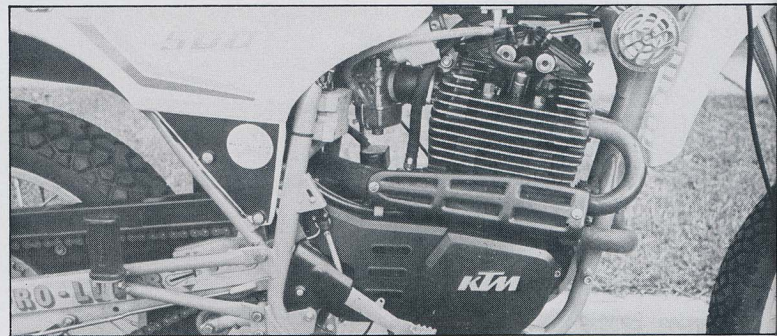
ABOVE This Rotax engine is identical to the XC version, but the factory geared it up to the sky. Various countershaft sprockets are available to suit your taste.
