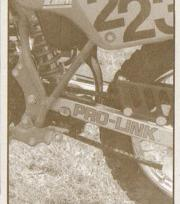
Pro-Link suspension is now fitted to the smallest of Honda's XR range. The short shock is mounted to the frame backbone and connected to the steel boxsection swingarm via the usual Pro-Link linkages.
