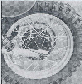
ABOVE Husqvarna have stuck with their 17" rear wheel decision on the larger bikes. More manufacturers have accepted the move and you now have a wider choice of tyres.
