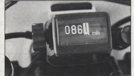
Odo has a magnified lens. Reset knob is large and easily reached while riding.
