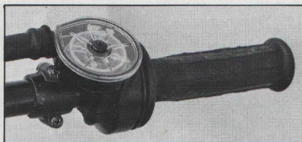
Clear top straight-pull throttle is gear driven. Lever brackets are easily changed without removing grips or throttle. Grips are good.
