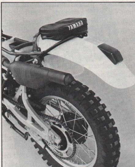
Tool bag is a nice shape and doesn't protrude past the top of the seat. Silencer is quiet and forestry legal. Fender has an integral tail light.
