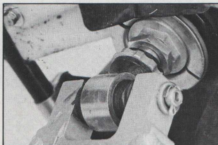
Shock rebound damping and spring preload are easily adjusted; the knurled ring adjusts damping, the double nuts adjust spring preload.
