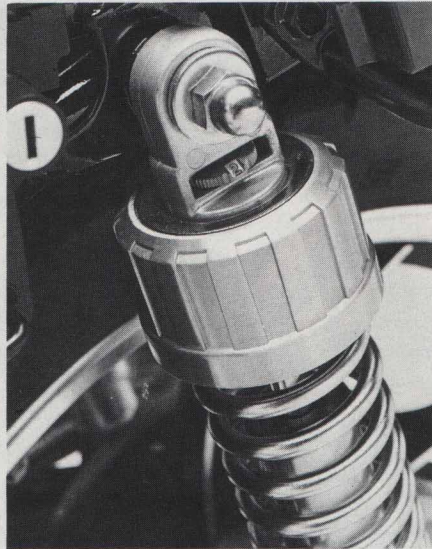
Stiff springs and useful four-way adjustable dampers give the Seca rear end a taut but controlled ride.
