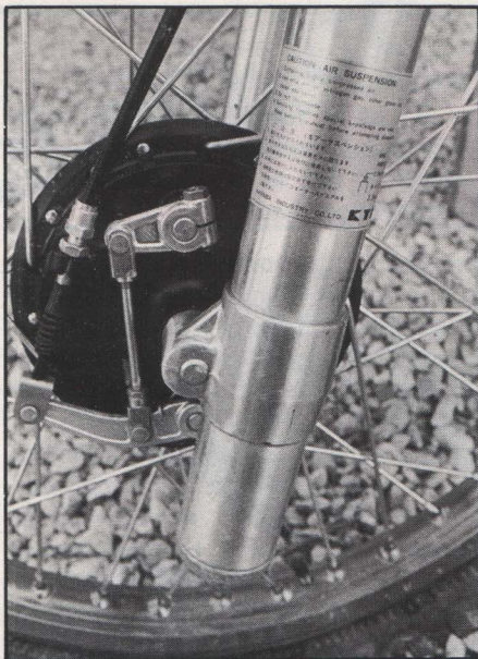
Leading axle forks and a powerful but smooth twin leading shoe front brake on the YZ250.
