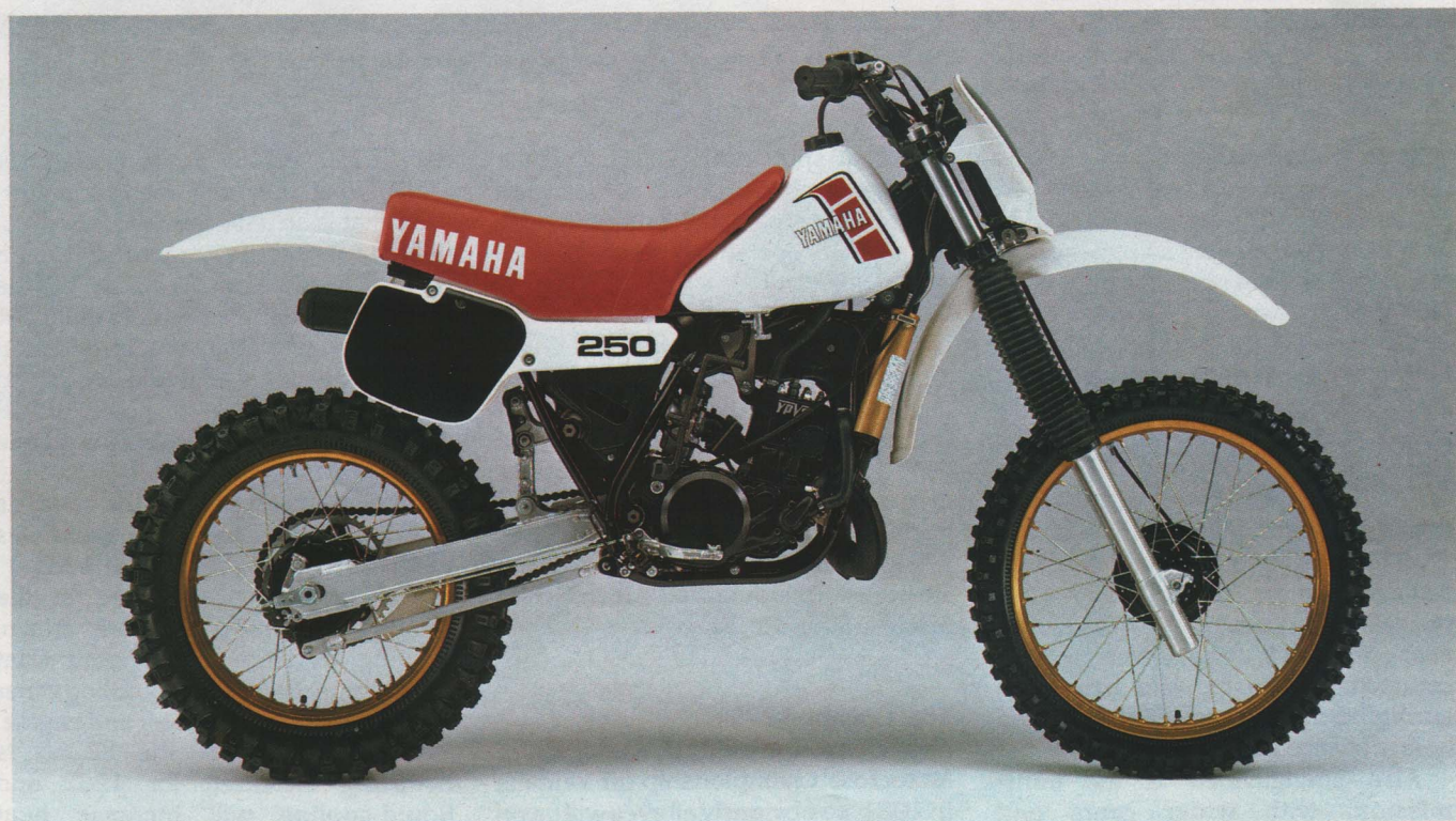
Also featured is the Yamaha Energy Induction System (YEIS). That little box beneath the gas tank gives much more mid-range power.
