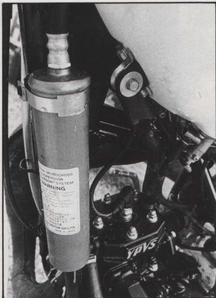
Remote reservoir for the gas damping of the monoshock suspension system.
