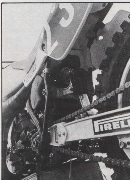
A plastic chain guide at the swinging arm pivot point on the YZ250's rising rate monoshock suspension.
