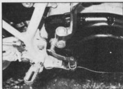
Rear brake lever (above) is shortened to protect it from rocks but makes brake less sensitive. 26mm carburettor (below) is set up for trials work with easily adjustable pilot screw with plastic cover and drain plug for float chamber.
