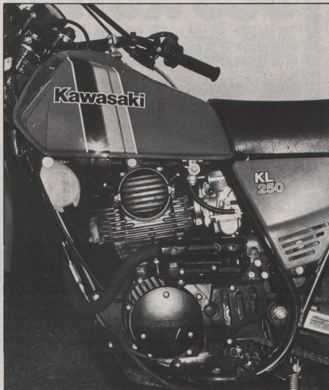
The Kawasaki's motor doesn't employ any form of balancing so it shakes a bit, but the constant vacuum carb ensures a smooth power delivery.
