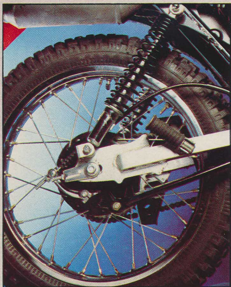
KE125 features painted box-section swinging arm and good guards
