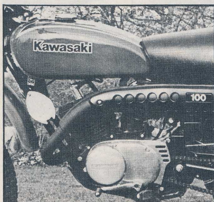
The disc-valve, two-stroke unit of the off-road styled KE100A9
